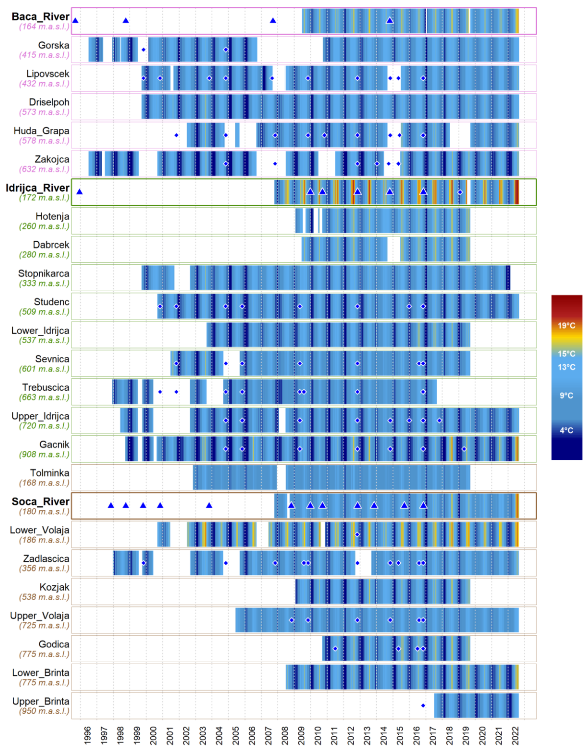
Figure 2. All recorded daily averages per site. Sites are color-coded according to their watershed (Bača, Idrijca or Soča), and classed per altitude. Floods that led to changes in the riverbed were noted in the field (blue diamonds) or identified from the maximum flows (see Figure 6; blue triangles).
